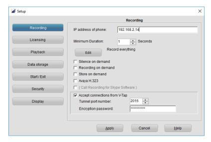
**NOTE1:** The PC's IP address must be entered as the "Tunnel Server Address" in the V-Tap unit.
