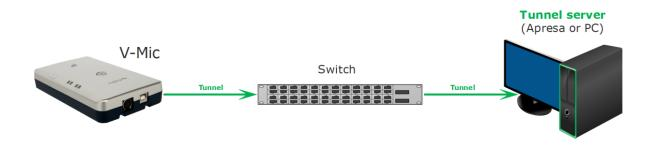
A connection between the V-Mic and the V-Archive PC software or an Apresa recorder is needed to get the recorded data automatically into a user accessible database.
