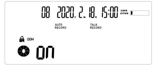
2. Press the Up/Down button to set the voice announcement function on / off (when the voice announcement is on, the OGM word on the home screen will be lit), ON means open, OFF means close
