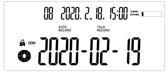
2. Press Up/Down/Left/Right key to select the date of the recording file, and press Enter to enter the playback mode
