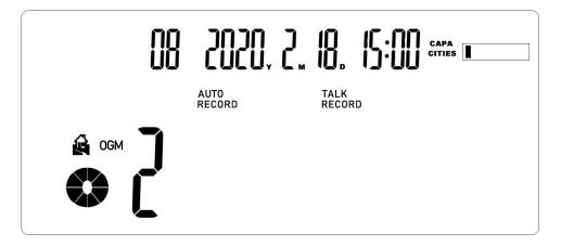
2. Press the Up/Down keys to set the number of ringing times for the message (0 means turn off the message function, 2-9 means ring times when the message function is on)
