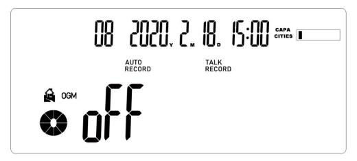
2. Press the Up/Down key to set, turn on/off the FSK incoming call automatic correction time
