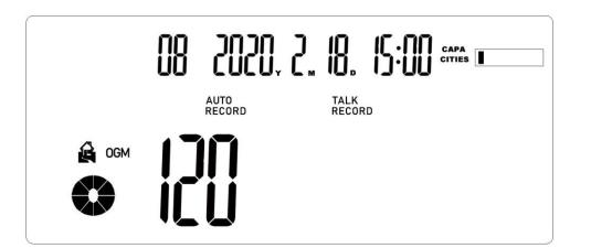
2. Press Up/Down/Left/Right to set the longest recording duration in sequence (1-120 minutes)
